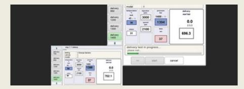
Improved metering capacity now allows to test up to 2000 mm3/Stroke fuel delivery. Therefore ED1029 CRH is capable to test both on-road and off-road Heavy Duty Common Rail Injectors at the same time.
